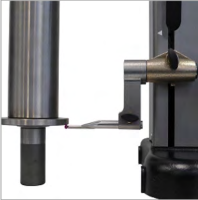
Height, thickness, and sequential measurement (TA-MI-101)
