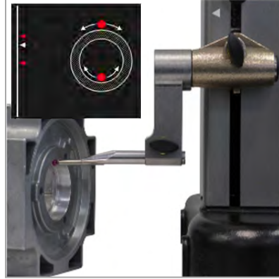
Diameter and centreline measurement with graphical help (TA-MI-101)
