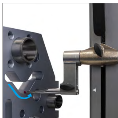
Perfectly steady measuring force guaranteed by the motorization (TA-MI-101)
