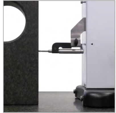
Perpendicularity measurements with electronic probe (TA-IH-126, TA-MS-101)
